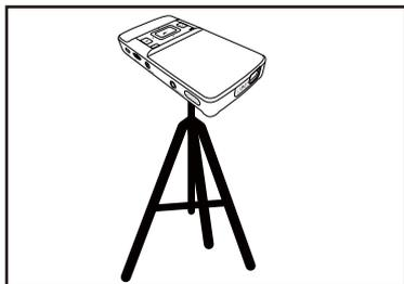
1. Screw a standard tripod into the screw hole on the projector.
